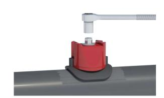
Correct tightening force indicator on strap mechanism
